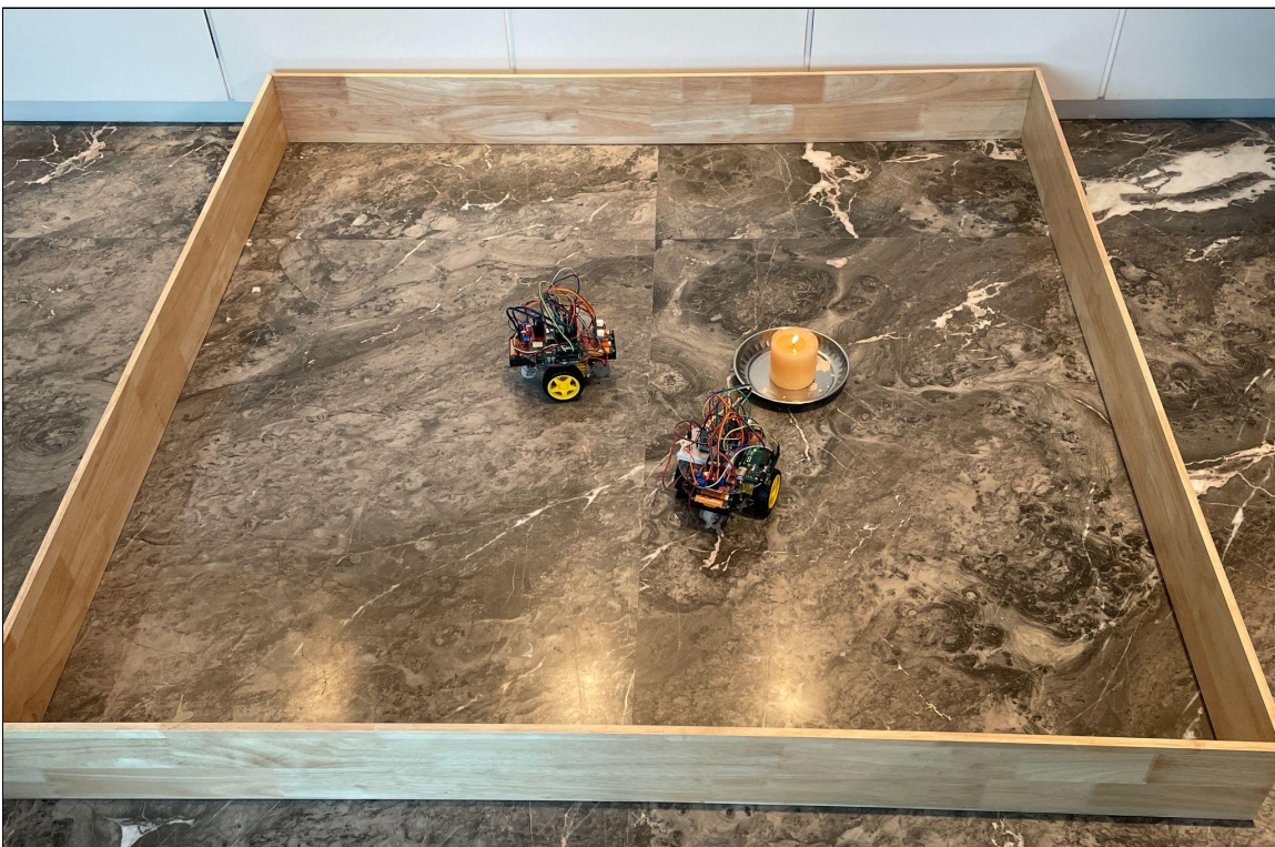
Figure 31: Two Swarm Robots Rendezvousing at Fire in Simulated Environment
